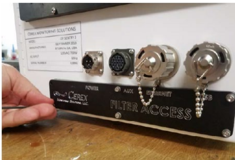
Figure A-5 . Location of filter access plate.
