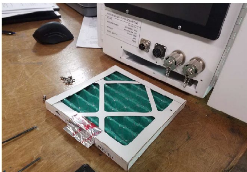
Figure A-7. Filter completely removed.
