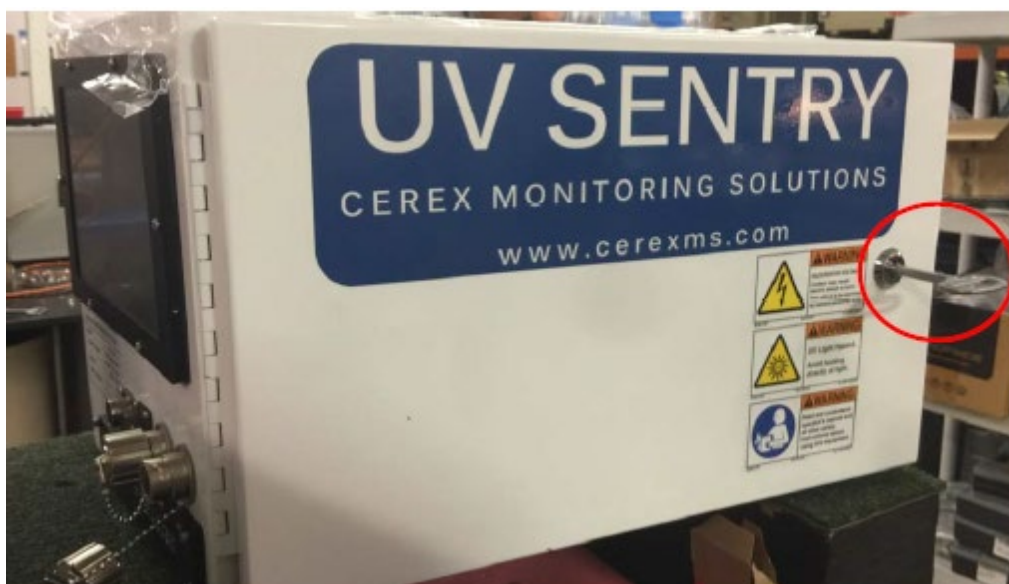
Figure A-9. Opening the source access panel.
